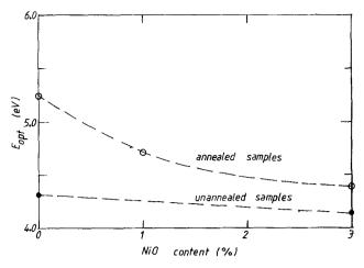
Figure 4 Variation of  $E_{opt}$  values with NiO content for unannealed and annealed glass samples.
