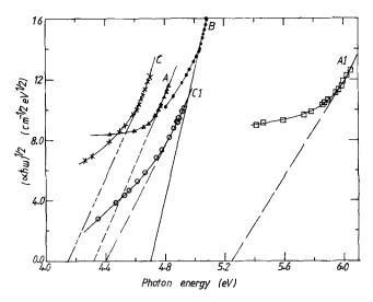
Figure 3 Absorption coefficient as a function of photon energy for unannealed and annealed glass samples (see Table I).
