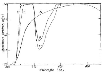
Figure 2 Absorption as a function of wavelength for annealed glasses (see Table I): Al (2.45 mm thick), B (1.35 mm thick), and Cl (2.00 mm thick).
