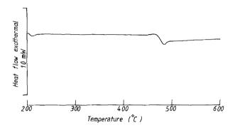
Figure 5 DSC curve of a sodium tetraborate glass sample doped with nickel oxide taken at a heating rate of  $10 \,\mathrm{K \, min^{-1}}$ .
